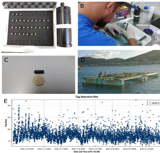
Fig. 1. (A) 30 accelerometer tags and 1 receiver, (B) seabream surgery to implant the tag, (C) tag size, (D) the experimental sea cage, (E) recordings for one fish over the monitoring period of 6 weeks.
