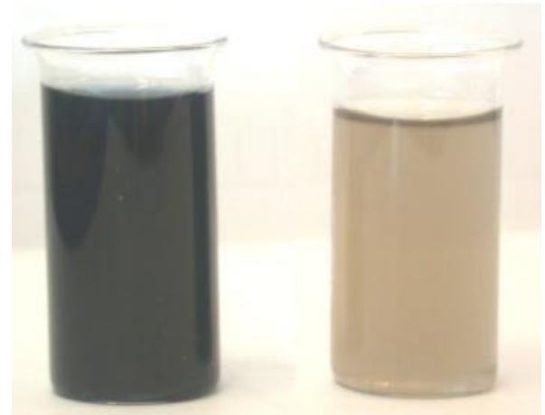
Photo: Textile effluent before (left) and after anaerobic treatment
